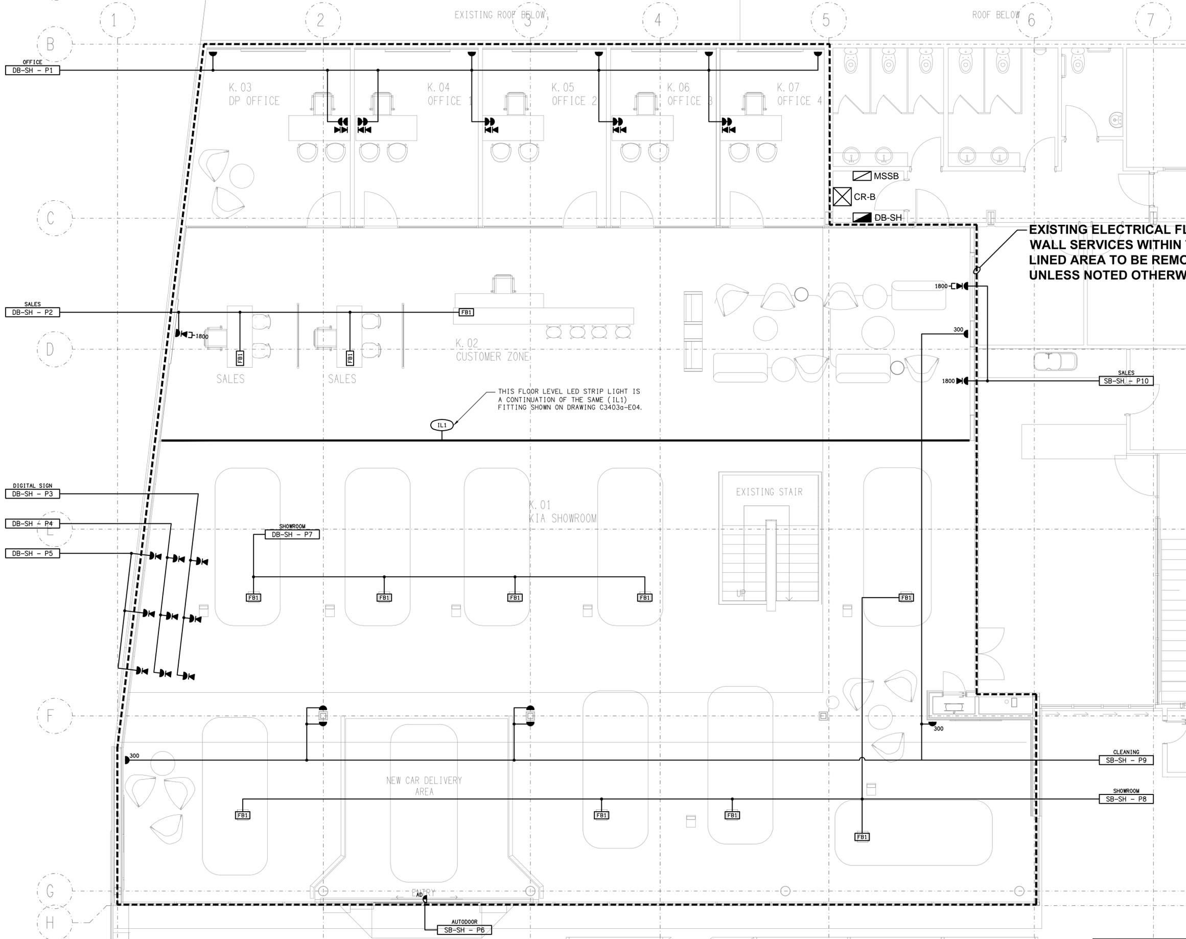
**EXISTING ELECTRICAL FLOOR & WALL SERVICES WITHIN THIS DASH LINED AREA TO BE REMOVED, UNLESS NOTED OTHERWISE.**
