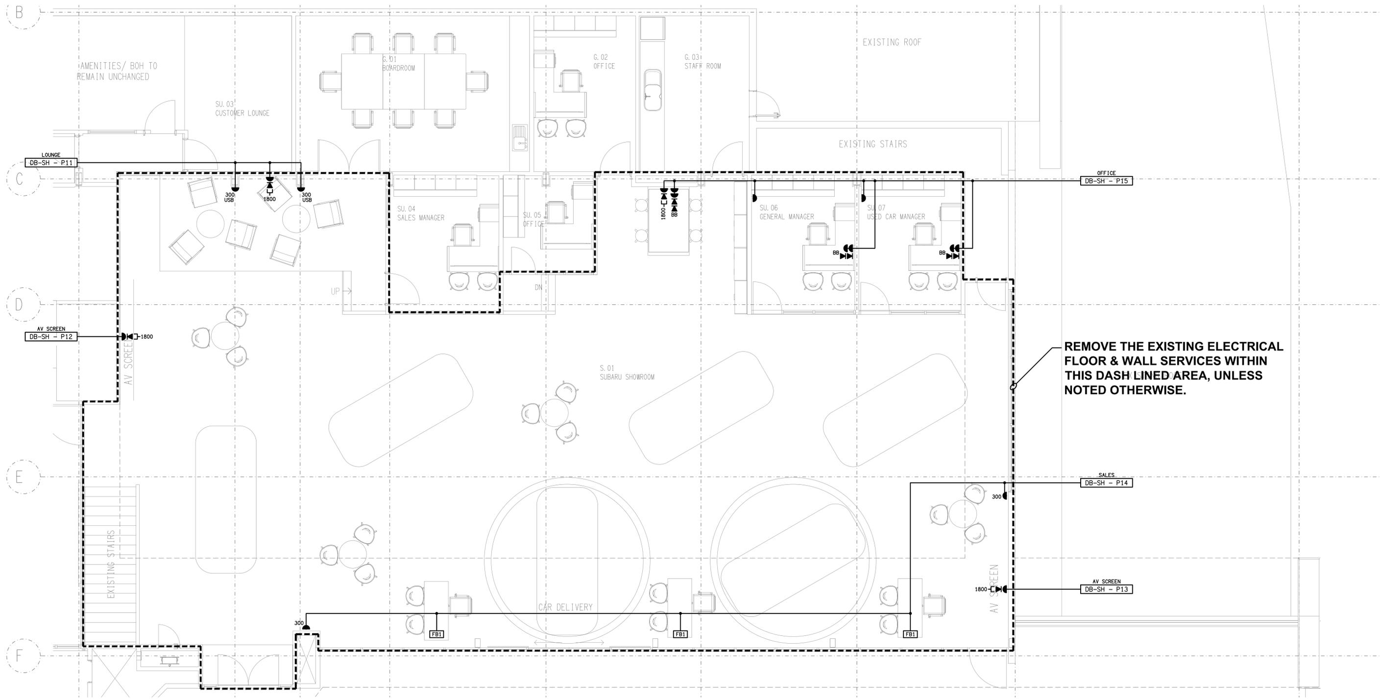
**REMOVE THE EXISTING ELECTRICAL FLOOR & WALL SERVICES WITHIN THIS DASH LINED AREA, UNLESS NOTED OTHERWISE.**
